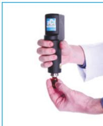
Our **automatic crimping tools** provide secure, reproducible crimps and quick removal of aluminum seals to and from all vials with crimp finish. The tools are ergonomically designed to reduce strain and arm injury associated with many manual crimping tools.
