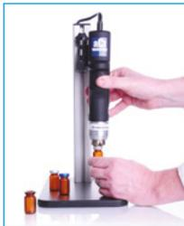
The **high performance crimping tool** is the fastest and most powerful WHEATON® crimping tool. It is strong enough for all steel and magnetic caps. Designed with external power source and cord (no battery). The high performance tool uses interchangeable jaw sets, so that you only need one tool and purchase the size crimper and decappers needed for your laboratory. This crimping tool has the ability to store up to nine separate programs for different caps and cap sizes.
