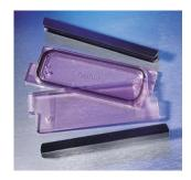
Corning<sup>®</sup> Hybridization Chambers are designed to hold microarray slides (25 x 75 mm) at constant humidity during hybridization incubations. The O-ring and retaining clips ensure that the reusable chambers remain watertight when submerged in waterbaths and airtight in hybridization ovens. Wells in the base hold 10 to 15  $\mu$ L of water to maintain optimal interior humidity.
