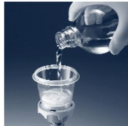
Place device onto a standard, #8 stopper, pour sample, and apply vacuum.
