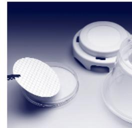
Place membrane onto solid or liquid medium and incubate. Discard the base. It's recyclable.
