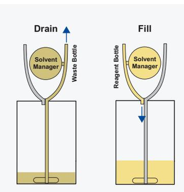
The reagents play an important role in the coulometric Karl Fischer titration. The Reagent Control keeps an eye on the important parameters so that once the maximum capacity is reached the user is prompted to replace the reagents. Contact with any of the reagents is avoided and the user always has an optimal system, ready to use and prepared to generate correct, repeatable results.
