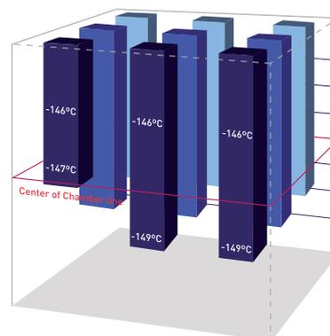
Comparison of temperature distribution in a liquid nitrogen freezer (vapour phase) and our MDF-C2156VAN mechanically refrigerated **Cryogenic** Freezer. The graph shows temperatures at different locations within the chamber.
