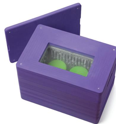
Freeze 2 CoolCell® LX cell freezing containers (up to 24 cryogenic vials) at collection site
