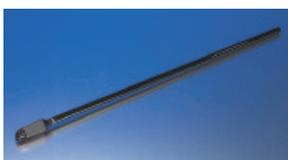
A simple air condenser, useful for condensation of materials with boiling points above 150°C, with an inner § 24/40 drip tip. Low actinic glass protects light sensitive materials.
