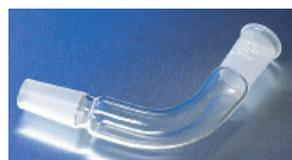
The arms are approximately 105° apart. One end is equipped with an outer ½ joint and the other end with an inner ½ joint of the same size. Used as a receiver adapter.
