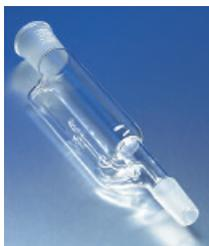
Bulb in siphon tube near the top of tube facilitates cycling of the siphoning action. The siphon tube is protected from accidental damage by the vapor tube. § joints at the top and bottom.
