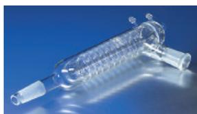
The Friedrichs type condenser affords very efficient operation. The helical inner tube fits closely within the jacket. The vapor tube is sealed to the jacket at an angle of 75° and has an outer ⌘ 24/40 joint.
