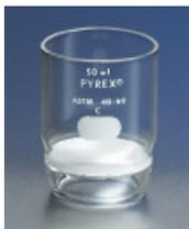
Particularly adapted to analytical work where precipitates are dried to constant weight at 110°C. Also suitable for higher temperatures, in which case it is advisable to heat in an electric furnace. Crucibles should not be subject to sudden temperature changes. In order to avoid strain, they should not be removed from the furnace until the temperature has dropped to 250°C. For low form, see Cat. No. 32960.
