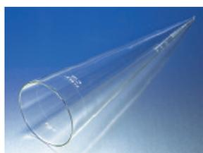
For determination of small amounts of suspended matter in sewage by the Imhoff Sedimentation Method. Graduated from 0 to 1 mL in 0.1 mL divisions, 1 to 10 mL in 0.5 mL and 10 to 40 mL in 1 mL; also marked at 1000 mL.
