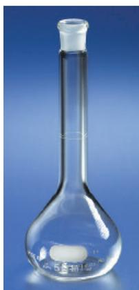
The strength of these flasks has been increased appreciably through machine-blown bodies to which are sealed heavy-beaded, heavy-tubing necks, tooled for polyethylene stopper. The stopper is made with a closed bottom and is of linear high density polyethylene to conform to § stopper dimensions. The graduation line is sharp and permanent and large white block letters make the inscription easy to read. The 2 mL size is test tube shaped.
