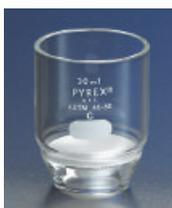
Particularly adapted to analytical work where precipitates are dried to constant weight at 110°C. Also suitable for higher temperatures, in which case it is advisable to heat in an electric furnace. Crucibles should not be subjected to sudden temperature changes. In order to avoid strain, they should not be removed from the furnace until the temperature has dropped to 250°C. For high form, see Cat. No. 32940.
