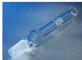
With one bulb and medium-sized  $\text{K}$  joints.
