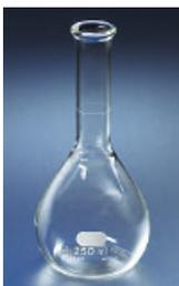
For use in determining phosphoric acid in mixed fertilizer. Of heavy construction throughout and with a wide neck.
