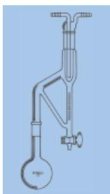
**3400 PYREX Brand, Volatile Oil Distilling Apparatus, Lighter Than Water, § Ground Joint**
