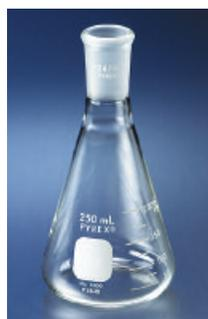
A range of Erlenmeyer flasks with joints. For convenience, these flasks are graduated to show approximate capacity.
