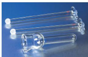
Supplied with two pestles to ensure dissociation of cells into fine particles with minimal damage to cell nuclei. Use the large clearance pestle for initial reduction of soft tissue. Complete the homogenization with the small clearance pestle. Particularly useful in enzyme studies where heat build-up must be avoided.
