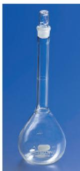
Calibrated to Class A tolerances in accordance with ASTM E-542 and E-288. Each flask is individually serialized and supplied with a Certificate of Identification and Capacity, traceable to NIST standards. The graduation line is sharp and permanent and large white block letters make the inscription easy to read. Supplied with a  $\text{F}$  stopper.
