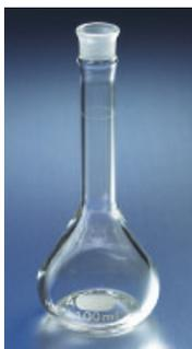
Designed for microchemical work. The heavy duty, wide mouth facilitates filling and mixing. Easy to read graduation line is sharp and permanent. Supplied with interchangeable standard taper ground glass stoppers.
