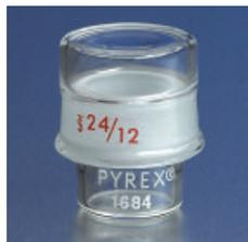
Joints Designed for use in weighing small samples. The closure style cap fits over the externally ground body.
