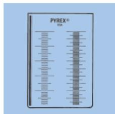
Used with oxidized sludge process for treatment of sewage and other wastes. 2000 mL heavy wall cylinder measures 5 1/8" I.D. x 7 1/2" high and is graduated in cc per liter, and in hundredths of a foot.
