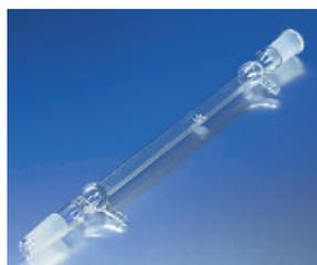
This condenser is designed with a heavy-wall outer jacket to provide a sturdy, long-lasting unit, while the inner tube has a thinner wall for efficient heat transfer. Tubulations are on the same side to reduce breakage. With the outer ⌘ joint at the top and the ⌘ inner joint at the bottom with a drip tip. The tubulation O.D. is approximately 10 mm.
