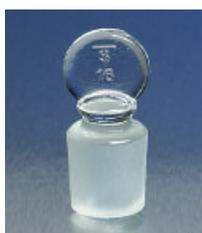
Pennyhead ₤ stoppers are generally used in flasks and separatory funnels.
