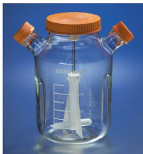
Baffled to enhance agitation of the contents of the flask. Dynamic Vortex impellers ensure high performance stirring. Center neck is 120 mm for ease in setup and cleaning. The wide 45 mm angled sidearms permit easier entry of 25 mL and 50 mL pipets for feeding and harvesting.
