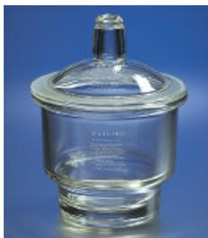
Designed for general analytical work. The large sturdy knob makes the cover easy to handle. Approximate bowl volume is 2200 mL. Not for vacuum applications.
