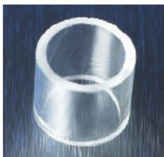
Clone a single cell or group of cells by surrounding them with this glass cylinder. Dip the end of the cylinder into a sterile silicone grease before pressing to the bottom of a culture flask to create an isolated well.
