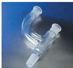
**9050 PYREX Brand, Connecting, Claisen Type, Three-Way, 3/4 Joints**
