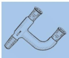
**9040 PYREX® Brand, Connecting, Claisen type, Three-Way, 3/4 Joints**
