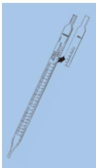
These shorty pipets, calibrated “to deliver” with blow-out, are ideal for use in confined areas. The 5, 10, and 25 mL sizes have tooled tops and the 50 mL has a polypropylene top end. Negative graduations on each pipet make it applicable for both serological and measuring procedures. Packaged in plastic bags so several can be removed without contaminating the entire pack. I.S.O. color-coding is printed directly on the tear strip.
