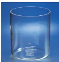
These jars are mold-blown with substantial walls for mechanical strength. The open end of the jar is ground flat. These jars can also be used as animal jars. Do not use with heat, pressure, or vacuum applications.
