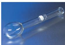
Flask, without tooled neck, is suitable for multiple micro digestions. Care must be taken to ensure the bottoms of the flasks do not come in contact with the heating elements. Most Kjeldahl equipment manufacturers have ring supports for this purpose.
