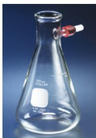
This filtering flask is a standard PYREX brand heavy wall filtering flask with a quick-release connector designed to accommodate 1/4" ID tubing, not included. For convenience, the flasks are graduated to show approximate capacity.
