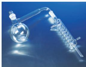
A general purpose batch distillation assembly with the facility for addition via the PYREX stoppered neck. Ideally suited for the batch production of high purity distilled water. The flask has a flat bottom with a side delivery tube, terminating in a joint. Graham condenser tubulations are 10 mm O.D.
