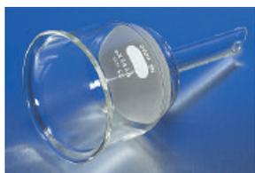
These funnels are suitable for vacuum filtration; however, the translucent plate should not be subjected to a pressure differential in excess of 1 atmosphere. The clear glass bodies afford visual examination during use and cleaning. The size number indicates filter paper diameters in millimeters.
