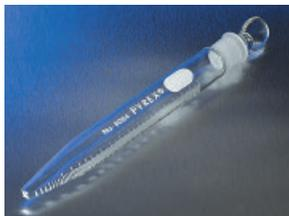
These tubes have white enamel graduations. The 5 and 15 mL sizes are graduated upward from the tip in 0.1 mL divisions. The 50 mL size is graduated upward from tip to 10 mL in 0.5 mL divisions, and from 10 to 50 in 1 mL divisions. The pennyhead stopper is solid.
