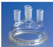
Cover has sturdy wall and a tooled flat flange at bottom which has a groove in the face to take an O-ring for a greaseless tight seal. Center neck and three side necks are 120° apart. All four necks have full length  $\text{F}$  outer joints. Viton® O-ring must be ordered separately.
