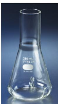
Delong style, with three baffle indents designed to provide greater agitation of solutions to improve oxygen or gas transfer when used with rotary or reciprocating shakers. Long neck reduces splashing and is designed for two-position polypropylene closures.
