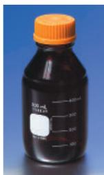
Heavy duty bottle of low actinic glass for use when storing/transporting light sensitive materials. Includes a linerless, one-piece, autoclavable, orange polypropylene, plug-seal cap with drip-free pouring rings. Glass bead indicates full capacity line. Permanent white enamel graduations and marking spots. Thread size: GL45. Neck I.D.: 29 mm I.D.
