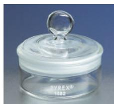
Low form bottle with a ST joint style opening that accepts a closed bottom hollow Pennyhead style stopper.
