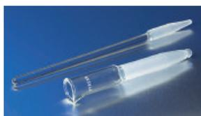
Designed to handle both initial grinding and final homogenization in the same sequence of operations. The lower conical section is intended primarily for the initial grinding. To assist in this work the clearance between mortar and pestle can be adjusted at will by raising or lowering the pestle. The upper cylindrical section is for the final homogenization.
