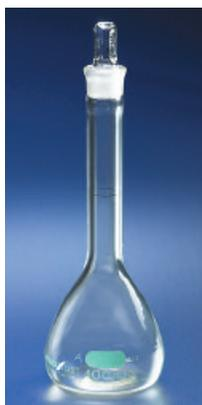
Flask features a protective PVC coating for longer product life and safety. Protective coating helps prevent glass from shattering and reduces spills. Autoclavable (121°C) and resistant to thermal shock. The graduation mark is easy to read. Supplied with § PYREX stopper.
