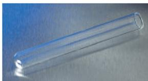
These one-use culture tubes are packaged for your convenience in easy-to-open, easy-to-use packs. The three small sizes come in a dispenser arrangement, and the larger sizes are bulk-packed. Made of borosilicate glass to reduce pH changes and contaminants potentially leached from soda-lime glass.
