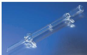
This condenser is designed with a heavy-wall outer jacket to provide a sturdy, long-lasting unit, while the inner tube has a thinner wall for efficient heat transfer. The tubulations are on the same side to reduce breakage and the adapter ends are all tooled for No. 3 rubber stopper fit. The tubulation O.D. is approximately 10 mm.
