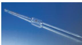
Calibrated to Class A tolerances in accordance with ASTM E-542, and ASTM E-969. Each pipet is individually serialized and supplied with a Certificate of Identification and Capacity, traceable to NIST standards. Sizes 1mL through 25mL are color-coded with colored graduations enameled onto the glass.
