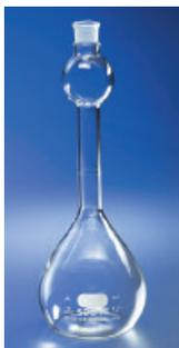
The upper bulb, located between the stopper and the capacity graduation is approximately one-tenth the flask rated capacity. The 2L size upper bulb is only one-twentieth capacity. The additional bulb assists in the mixing of liquids or powders when shaken.
