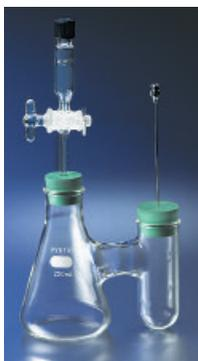
Used to measure production of carbon dioxide produced by microorganisms grown on a variety of culture medium over longer periods of time. Minimizes the need for commonly used gas trains. Also useful in Bioremediation studies. Supplied complete with #6 rubber stopper in flask neck #7 rubber stopper in the side tube and 16 ga. needle.
