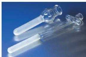
These 40 mL capacity PYREX homogenizers are designed for grinding small samples for pathological and biochemical work. The catch basin bulb has a 55mm outer diameter. Made in accordance with Federal Specification DD-T-363a. It may be used manually but is adaptable for use with a slow speed stirrer by means of a rubber stopper and a connecting rod.
