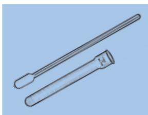
These tissue grinders (homogenizers) are used in preparing small samples for pathological and biochemical studies. Designed to be motor-driven. Use a friction clutch to eliminate damage to the pestle from pieces of connective tissue or muscle. The clearance between the ground tube and pestle is approximately 0.15 mm. The parts are ground to a medium grind to insure adequate abrasive qualities, yet deliver a fine homogenous sample.
