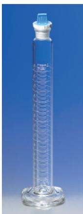
Calibrated “to contain.” Useful as a mixing cylinder. Graduations are in durable white enamel. Stopper made of linear, high density polyethylene, to conform to § stopper dimensions. The stopper has a ribbed top to provide a sure grip when inserting or removing.
