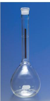
The capacity mark is a fine line etched through a narrow red band into clear glass, making a filler unnecessary and giving high legibility, accuracy and permanence. With § stopper. Calibrated “to contain.”
