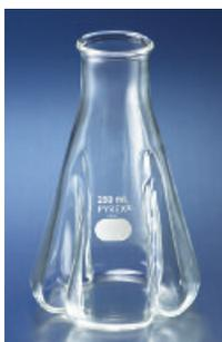
Flasks are used for converting homogenous tissue samples into cell suspensions by digestion of connective proteins. Heavy beaded neck accepts cotton plugs. Four extra-deep baffles enhance vigorous agitation.
