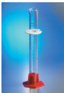
These PYREX VISTA cylinders are calibrated “to contain” (TC). They are supplied in two parts – a strong, accurate glass graduate and a detachable, sturdy plastic base which absorbs impacts and reduces breakage. Tolerances are  $\pm 5\%$  of total at any point. By removing the base, the graduate can be conveniently stacked. Bumper guards are supplied with 2 5mL through 100 mL inclusive. The 10 mL has a funnel top for careful pouring. read. Snap caps are supplied with all sizes.
