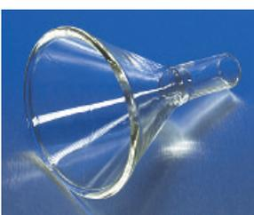
With a short stem. For use in transferring powders or filling bottles.
