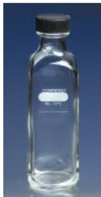
Narrow mouth bottle with a cut-line graduation mark at 99 ± 1 mL. Phenolic cap with rubber liner will withstand sterilization (wet at 121°C). Meets the requirements for milk dilution bottles stated in the *Standard Methods for the Examination of Dairy Products*, published by the American Public Health Association.
