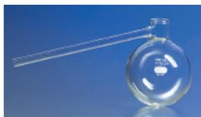
For the distillation of bituminous materials suitable for road treatment. Also used in the *Standard Method of Test of the Distillation of Creosote Oil*, American Wood Preservers Association, method 11e, Barrett method C 9, American Association of State Highway Officials, methods T 52 and T 62.
