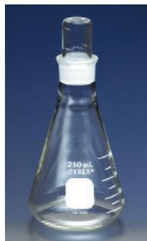
For convenience, these flasks are graduated to show approximate capacity. The 25, 50 and 125 mL flasks are satisfactory for use as a weighing bottle.
