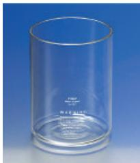
Recommended for use as animal jars or for other purposes where resistance to hot air and steam sterilization is of importance. These jars are blown with walls approximately 4.5 mm (3/16") thick. The open ends are finished with a fire-polished bead to increase mechanical strength. Jars listed under Cat. No. 6942 can also be used as animal jars. Do not use with heat, pressure or vacuum applications.
