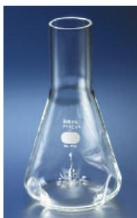
Delong style neck, with three extra-deep baffles, to enhance gas transfer when used with rotary or reciprocating shakers. Long neck reduces splashing and is designed for two-position polypropylene closures. Closures are sold separately.
