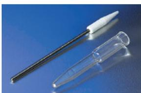
Recommended for soft tissues found in the liver and brain. Designed to handle both initial grinding and final homogenization in the same sequence of operations. Mortar is unground and the pestle contact surface is PTFE, threaded onto a stainless steel shaft.
