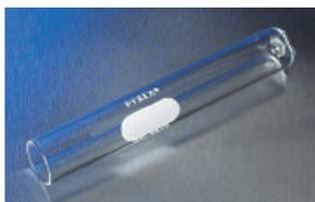
Rimless for greater convenience in plugging and rack storage. Walls and bottoms are of uniform thickness. Ends are fire-polished. The 6, 22, and 25 mm O.D. tubes do not have marking spots.
