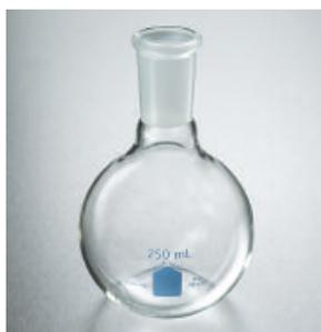
These PYREX VISTA flat bottom boiling flasks have full length outer 24/40  $\text{F}$  joints, but with shorter necks. Wall thicknesses are controlled to provide balance between thermal expansion and mechanical strength for greater shock resistance. The flat bottom boiling flasks are designed to ASTM E-1403. Adapter Cat. Nos. 8800, 8820 and 8825 are used to connect flasks with different size joints, thus allowing numerous combinations for diverse assemblies.
