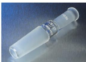
With an outer  $\text{K}$  joint at the top and a larger inner  $\text{K}$  joint at the bottom.
