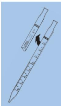
These shorty pipets, calibrated “to deliver” with blow-out, are ideal for use in confined areas. The 5, 10, and 25 mL sizes have tooled tops and the 50 mL has a polypropylene top end. Negative graduations on each pipet make it applicable for both serological and measuring procedures. I.S.O. color coding is printed directly on the Steri-View wrapper.
