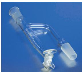
For determining water content in petroleum or bituminous products, graduated upwards from the stopcock to 3 mL in 0.2 mL divisions, and from 3 mL to 20 mL in 0.5 mL divisions. Reference: Barrett method B-2. Also can be used as Dean Stark distillation apparatus specified in British Standard 756, but utilizes a common U.S. ground joint. It is also an optional setup for ASTM D-95.
