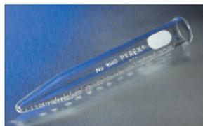
Of heavy wall construction, for greater mechanical strength, with durable, white enamel graduations. The 12 mL size is graduated upward from tip in 0.1 mL divisions. The 40 mL size is graduated in 0.5 mL divisions to 10 mL, and from 10 to 40 mL in 1 mL divisions.
