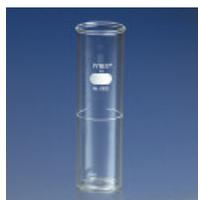
Single line encircles the jar at a point approximately 51 mm above the bottom to assist in measuring the sample. Reference: ASTM D-97, D-1500, D-2500.
