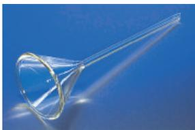
These funnels have a beaded edge for strength. They are fabricated from blanks formed to a 60° angle, which permits accurate fitting of the filter paper, thus reducing filtering time. The stems are made of heavy wall tubing approximately 150 mm (6") long.
