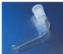
The arms are approximately 105° apart. The upper end is equipped with an outer ½ joint. The lower end is cut off at an angle and is used as a receiver adapter. Tube O.D. is 12 mm.
