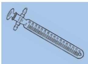
The manometer tube is enclosed in a round bottom, graduated jacket and is sealed to a stopcock plug. T-sidearm permits drawing and venting the vacuum. In use, mercury is placed in the inner tube and in the jacket bottom to measure the pressure differential. The legible red scale ranges from 0 to 160 mm. Not recommended for positive pressure. Mercury filling instructions are supplied with each instrument. Uses 5 to 6 mL mercury. Mercury not supplied.
