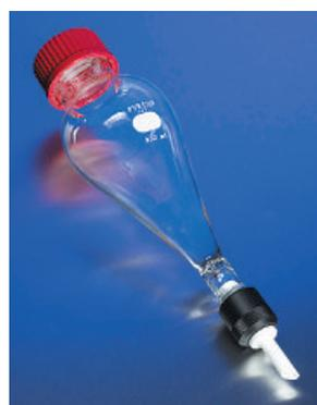
Improved Squibb type separatory funnel provides an unbreakable, all PTFE, valve and drip tip and has a screw thread closure at the top. Supplied complete with PTFE valve assembly and screw cap with PTFE faced silicone liner.
