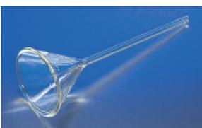
Have a strong beaded edge. These funnels are fabricated from blanks formed to a 60° angle. In addition, they have depressed inside flutings which further decrease filtering time.
