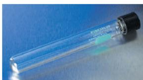
Tube features a protective polymer coating for longer product life and safety. Protective coating helps prevent glass from shattering and reduces spills. Autoclavable (121°C) and resistant to thermal shock. Furnished with deep-form phenolic caps to facilitate handling and sealing. Caps are resistant to autoclaving and feature glued-in, white rubber liners.
