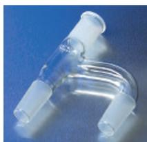
The PYREX brand solvent recovery head allows for condensation and collection of solvents while performing concentrations with a Kuderna-Danish concentrator. 96-99% solvent recovery allows for concentrations to be done outside the hood. Unique, simple design allows use with existing condensers and flasks.
