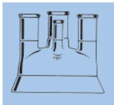
Cover for flask Nos. 5370 and 5380. Center neck and three side necks, all with full length § outer joint. Two of the side necks are 180° apart, while the third one, with a § 10/30 joint, is equidistant from the other two. The bottom cover has inside diameter of 4 inches (approx. 100 mm), and has a tooled portion at the end to obtain a thickened outwardly tapered finish with finely ground flat bottom.
