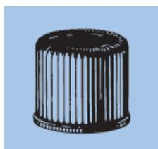
This cap is fabricated of a resin specially formulated to resist the effects of temperature and steam in autoclaving. Caps are provided with a glued-in rubber liner over which is firmly bonded a Teflon interface which provides a highly inert sealing face.
