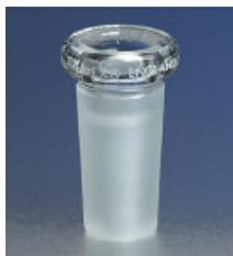
These adapters are fabricated with heavy walls for mechanical strength and are further strengthened by the heavy, uniform rim at the top which affords a serviceable finger grip. These adapters are shorter than the conventional type, thus allowing more compact and convenient assemblies. Useful for attaching ½ thermometers.
