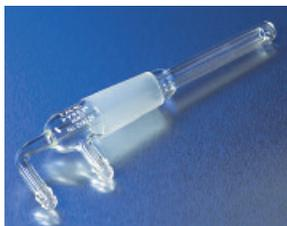
A simple condenser, of relatively low efficiency, often used to regulate refluxing by adjusting the flow of air or water through it (dephlegmation). The tubulation O.D. is approximately 10 mm.
