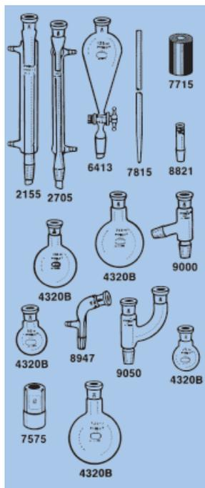
Similar to Cat. No. 6949, as many of the same standard laboratory experiments can be performed with this kit. It includes a distillation column and bleed tube for steam distillation or gas flow reactions. The components of the kit are held in foam within a polyethylene case. The overall case size is approximately 130 mm x 256 mm x 343 mm. For more detail on individual components of the kit and available parts, refer to the specific catalog numbers.
