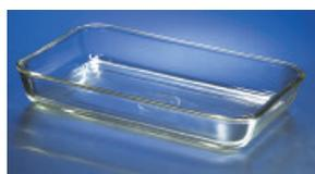
This tray will withstand hot air or steam sterilization. Useful for gel work or paper chromatography. Do not place over direct heat, for oven use only.
