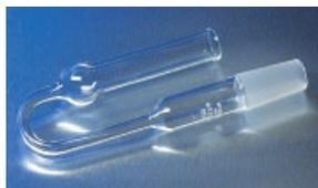
Inverted form with the inner  $\text{K}$  joint at one end only, with a single bulb. The chamber is approximately 110 mm long including the bulb, 30 mm O.D. and will take a No. 2 rubber stopper.
