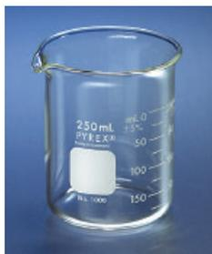
Beaker, with spout, manufactured with uniform wall thickness, offers optimum balance between thermal shock resistance and mechanical strength. For convenience, the 250 through 4000 mL beakers have a double graduated metric scale to indicate approximate content. All sizes have an extra large marking spot. The 10 mL size is not graduated.
