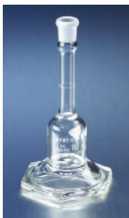
Calibrated to Class A Tolerance and individually serialized and supplied with a Certificate of Identification and Capacity. To improve the stability of this flask, a hexagonal base has been added. The graduation line is sharp and permanent and the white markings are easy to read. Each flask features a PYREX stopper.
