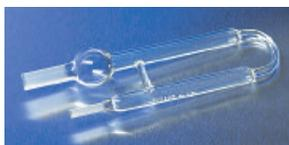
PYREX purge and traps glassware is designed for use in Tekmar® purge and trap equipment.
