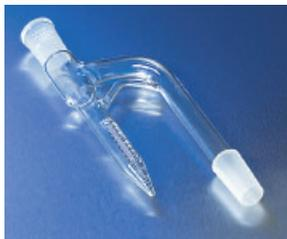
For determining water by distillation. Receivers have a § 24/40 ground joint on the sidearm. The 10 mL receiver is graduated, from 0 to 1 mL, in 0.1 mL intervals, with a maximum scale error of 0.05 mL. Graduation intervals from 1.0 to 10.0 mL are 0.2 mL, with maximum scale error of 0.1 mL. The 25 mL receiver is graduated, from 0 to 1 mL, in 0.1 mL intervals, with a maximum scale error of 0.05 mL. Graduation intervals from 1.0 to 25.0 mL are 0.2 mL, with a maximum scale error of 0.1 mL.
