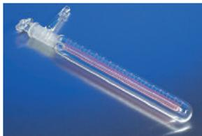
The manometer tube is enclosed in a round bottom, graduated jacket and is sealed to a stopcock plug. In use, mercury is placed in the inner tube and in the jacket bottom to measure the pressure differential. Not recommended for positive pressure. The legible, red scale ranges from 0 to 160 mm. Mercury filling instructions are supplied with each instrument. Uses 5 to 6 mL mercury. Mercury not supplied.
