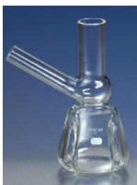
Delong style neck on flask and sidearm to accommodate plastic closures. Designed with a well below the sidearm to prevent unseparated tissues from being poured out of the flask. Four extra long, extra deep baffles promote vigorous agitation. Flasks are used for converting homogenous tissue samples into cell suspensions by digestion of connective tissues.
