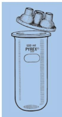
The 500 and 1000 mL kettles have interchangeable covers with four openings to accommodate 24/40  $\text{F}$  joints. Kettles of 2000, 3000, and 4000 mL capacity have interchangeable covers and have openings to accommodate three  $\text{F}$  24/40 joints and one  $\text{F}$  34/45 joint. Interchangeable  $\text{F}$  joints allow quick assembly with condensers, stirrers and funnels. Flanges of covers and bottoms are finely ground for a tight seal. For use with heating mantle only.
