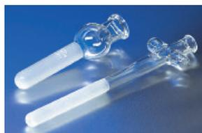
These grinders are designed for use in hand grinding small samples for pathological or biochemical studies. It may also be motor driven at low speed if some form of friction release is provided. The mortar tubes and pestles are ground to be interchangeable. Clearance between the two parts is approximately 0.15 mm. The medium grind provides the required abrasive action to deliver well homogenized samples. Made in accordance with Federal Specification NNN-T-360B.
