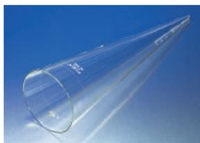
For use with heavy sediments, where ability to read small volumes is unimportant. Graduated from 0 to 1 mL in 0.1 mL divisions, 1 to 10 mL in 0.5 mL and 10 to 40 mL in 1 mL; also marked at 1000 mL. The blunt tip increases its ruggedness and cleaning ease.
