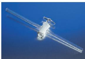
Closely controlled grinding techniques allow this general use stopcock to be used at pressures down to 10<sup>-4</sup> torr (mm Hg) when correctly greased. For additional strength, sidearm seals are heavy and uniform.
