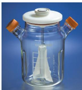
Baffled to enhance agitation of the contents of the flask. Dynamic Vortex impellers ensure high performance stirring. Extra-wide center neck is 140 mm for ease in setup and cleaning. The wide 45 mm angled sidearms permit easier entry of 25 mL and 50 mL pipets for feeding and harvesting. Unique Shur-Lok® cap design on center neck has a compression gasket to ensure a tight seal of the flask that can be visually confirmed after autoclaving.
