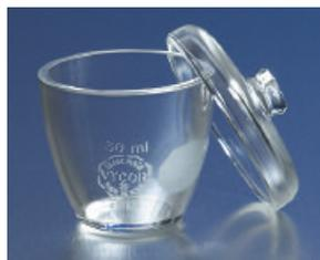
The transparent body and lid are useful in analytical work, particularly where ashing of the sample is required. Lids will be found useful for covering platinum or opaque crucibles. Note: Using covers of dissimilar material can cause spalling.
