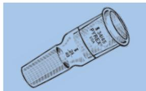
With an outer  $\text{K}$  joint at the top and a smaller inner  $\text{K}$  joint at the bottom.
