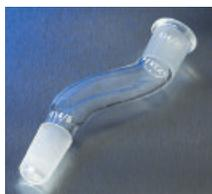
With ½ outer joint on one end and ½ inner joint on other end. Joints are the same size on both ends.
