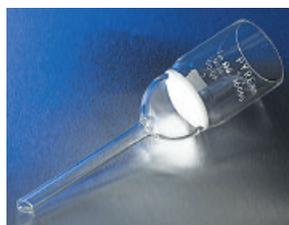
These funnels are especially useful where filter paper would be attacked by the material being filtered. The disc should not be subjected to pressure differential in excess of 1 atmosphere. The top edge is beaded.
