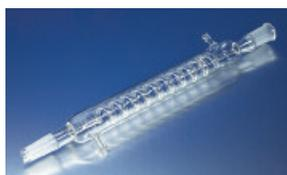
This condenser has a high surface area per unit length of jacket. Primarily used in vacuum distillations. With the outer joint at the top and the inner ⌘ joint at the bottom with a drip tip. The tubulation O.D. is approximately 10 mm.
