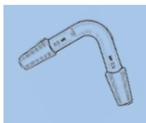
The arms are approximately 75° apart and both are equipped with inner ½ joints of the same size. Often used as a stillhead adapter
