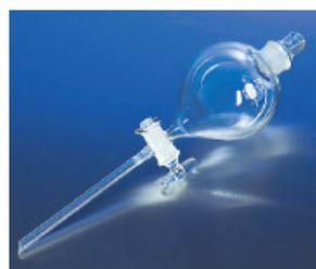
These funnels are made from specially molded blanks which are tapered toward the stopcock to facilitate the separation of liquids. Their sturdy design makes them excellent for rack work.
