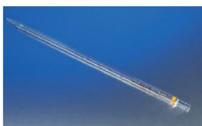
Calibrated to Class A tolerances in accordance with ASTM E-542, and ASTM E-1293. Each pipet is individually serialized and supplied with a Certificate of Identification and Capacity, traceable to NIST standards. Calibrated “to deliver” their total capacity without blow-out. Color-coded by size for easy identification. Colored graduations are enameled onto the glass. The top end of 5 to 25 mL sizes is constricted (Mohr type).
