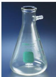
Flask features a protective PVC coating for longer product life and safety. Protective coating helps prevent glass from shattering and reduces spills. Autoclavable (121°C) and resistant to thermal shock. For convenience, the flasks are graduated to show approximate capacity. Tubulation O.D. is 10mm on sizes up thru 1000 mL. Tubulation O.D. is 12.5 mm on 2000 and 4000 mL sizes. The tubulation is not coated to allow easy connection of standard size tubing.
