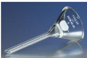
This type is very useful in preparation work, or in making separations where it is necessary to wash the precipitate and redissolve with chemicals which would attack filter paper. The angle of the funnel body facilitates the removal of precipitates.
