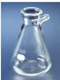
These small filtering flasks are recommended for microchemical use. All flasks have permanent white enamel marking spots.
