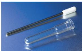
Homogenization occurs as the sample and buffer are forced through the cylindrical portion of the mortar as the pestle is rotated downward. Mortar is unground and pestle contact surface is PTFE, threaded onto a stainless steel shaft.
