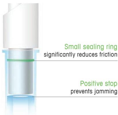
The Rainin LiteTouch System dramatically reduces the amount of force required to load and eject tips. LTS pipettes work in concert with LTS tips to deliver a perfect seal every time.
