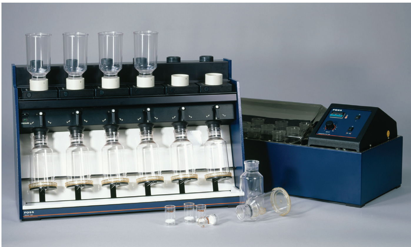
Semi-automated incubation and filtration system for quantitative determination of dietary fibre* in food, cereals, fruit and vegetables.
