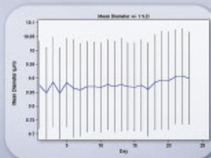
The Trend data function is used to plot statistics from a number of sample runs on one graph or report. This is useful in a process where a sample is measured at specific time intervals for example. These individual data files can then be used to create a Size Trend. These 'trend files' can be updated and added to as often as necessary.
