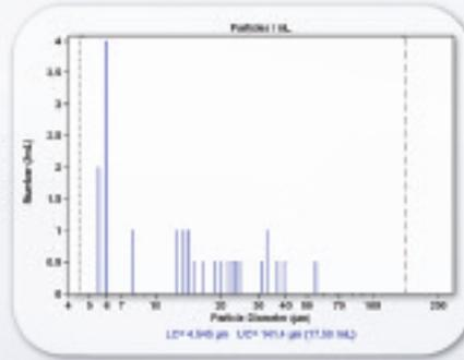
The determination of particle size and number is used to establish the level of insoluble material contaminating liquids. Usually the concentration of non-soluble contaminants is too low to be characterized with any other technology, but with the Multisizer 3 purification processes can easily be monitored.
