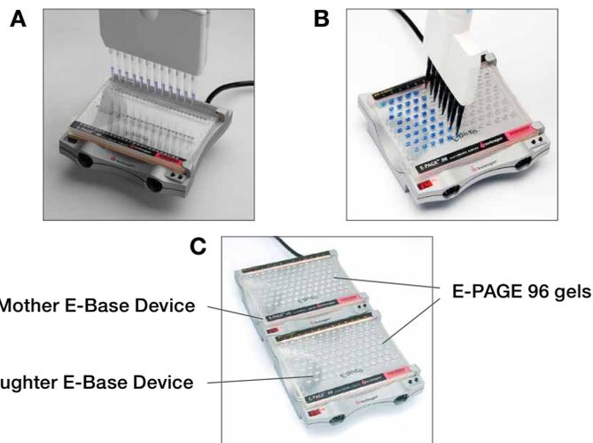
**Figure 23. Loading and running E-PAGE gels. (A)** Loading an E-PAGE 48 gel using a multichannel pipettor. **(B)** Loading an E-PAGE 96 gel using a multichannel pipettor. **(C)** The Mother/Daughter E-Base Device combination.
