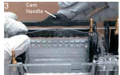
3. Place the cassette in the chamber with the wells facing towards you. Hold the cassette in a raised position and close the clamp by moving the cam handle forward.
