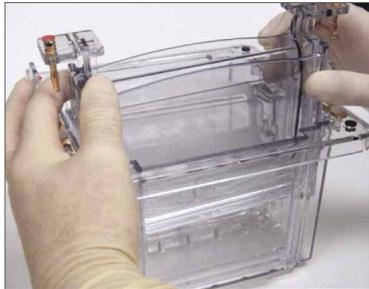
1. Insert the XCell4 SureLock Midi-Cell assembly in its unlocked position into the center of the midi-cell base. The XCell4 SureLock assembly slides down over the protrusion in the midi-cell base.
