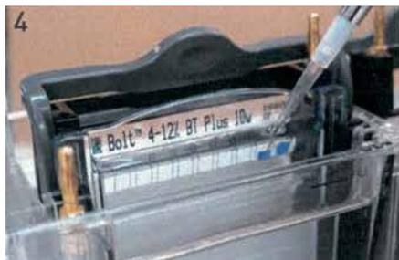
4. Make sure the wells are completely filled with 1X buffer. Load your samples and markers.
