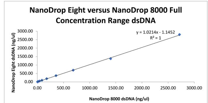
Figure 1: A linearity comparison between the NanoDrop Eight instrument versus the NanoDrop 8000 instrument across the entire concentration range for the sample dilutions. The regression line ( $R^2 = 1$ ) demonstrates that the NanoDrop Eight dsDNA concentration results were well aligned with the values obtained on the NanoDrop 8000 Spectrophotometer.
