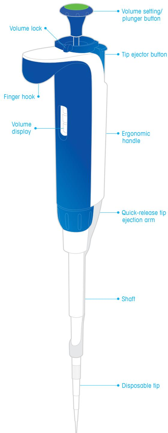
Figure 5. Air displacement pipette operation.
