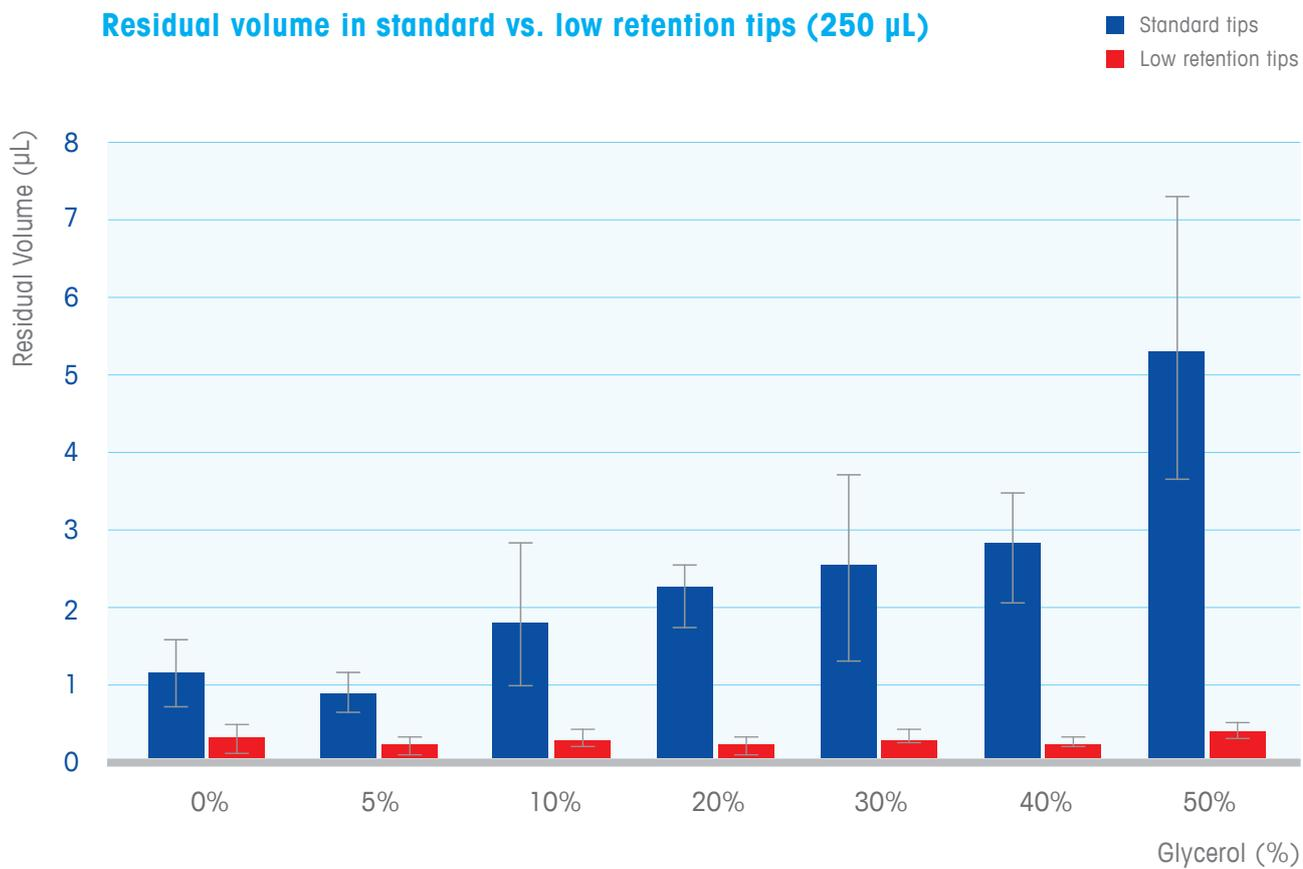
**Figure 10. Data indicates improved sample dispensing with low retention tips compared to standard tips when pipetting samples with increased viscosity (demonstrated by increased glycerol levels).** For reference, most thermostable DNA polymerases and many other enzymes are routinely suspended in buffers which contain 50% glycerol.
