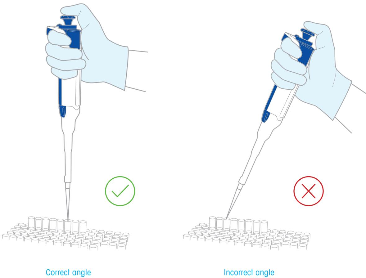
Figure 14. Correct vs. incorrect immersion angles.
