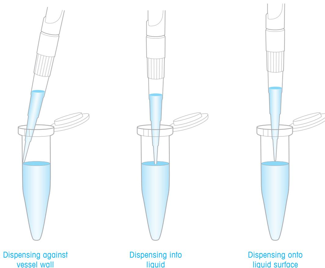
Figure 16. Consistent sample dispensing with good technique.
