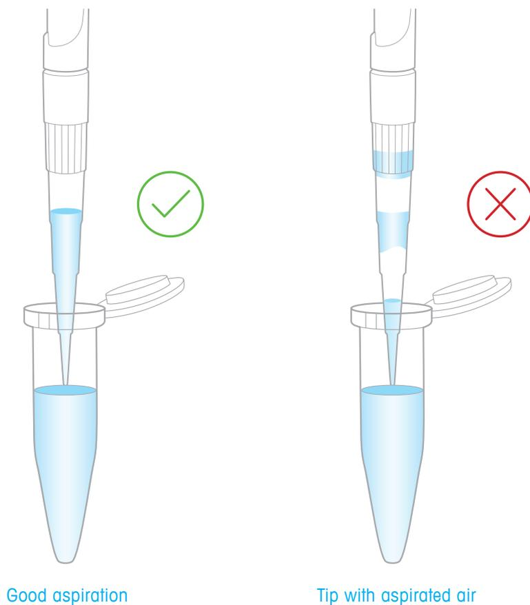
Figure 15. Aspiration using consistent pipetting rhythm avoids air gaps and bubbles.
