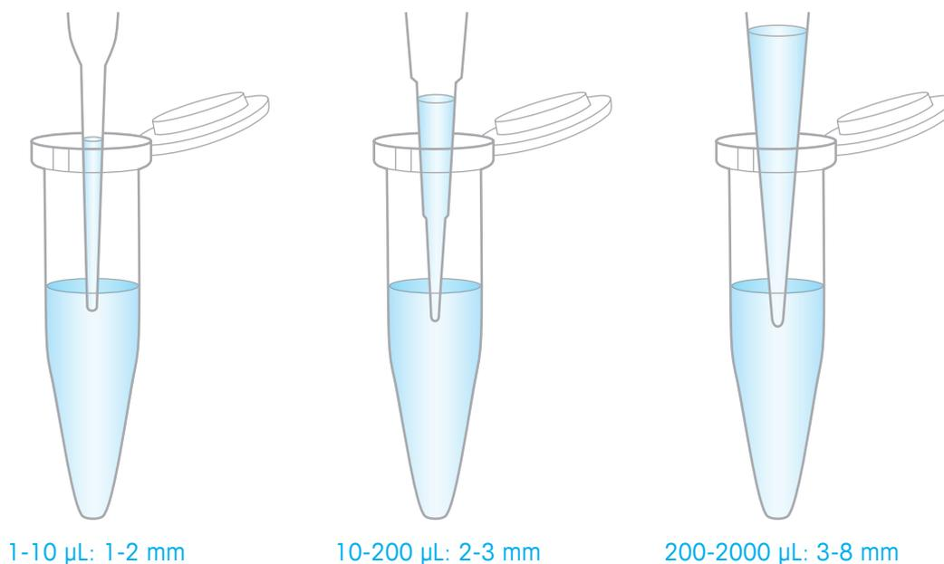
Figure 13. Tip immersion depths for 1 to 2000  $\mu\text{L}$  tips.
