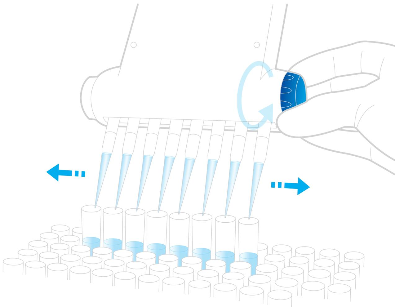
Figure 2a. Turning the spacing adjustment knob on a Rainin XLS Adjustable Spacer pipette to accommodate tube formats or wider spacing formats.
