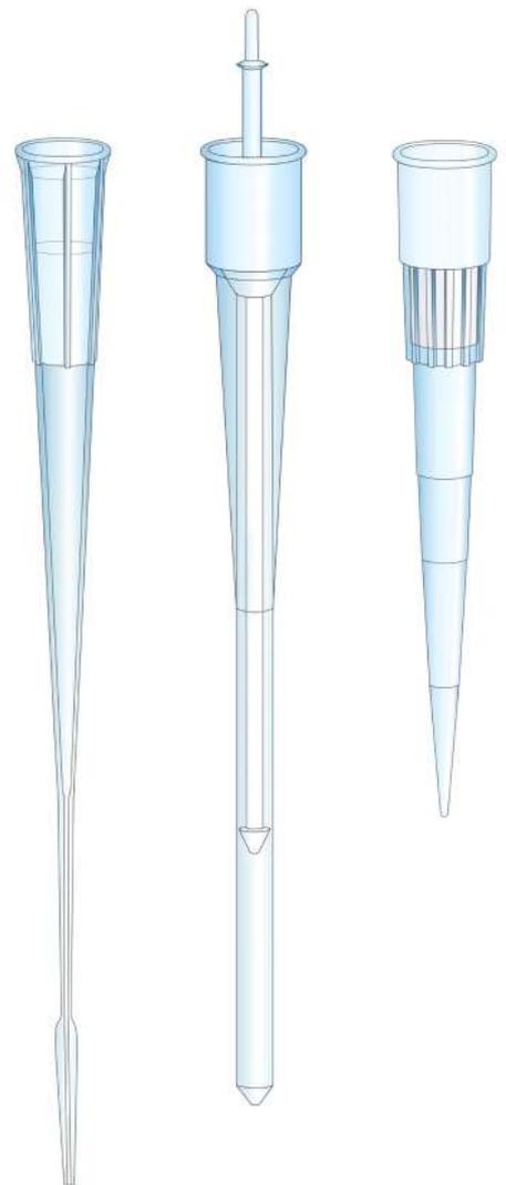
Capillary piston tips rely upon the movement of a piston within a capillary and generate greater force to deal with recalcitrant samples. The absence of an air gap also renders these tips a better choice for dealing with volatile organic liquids.
