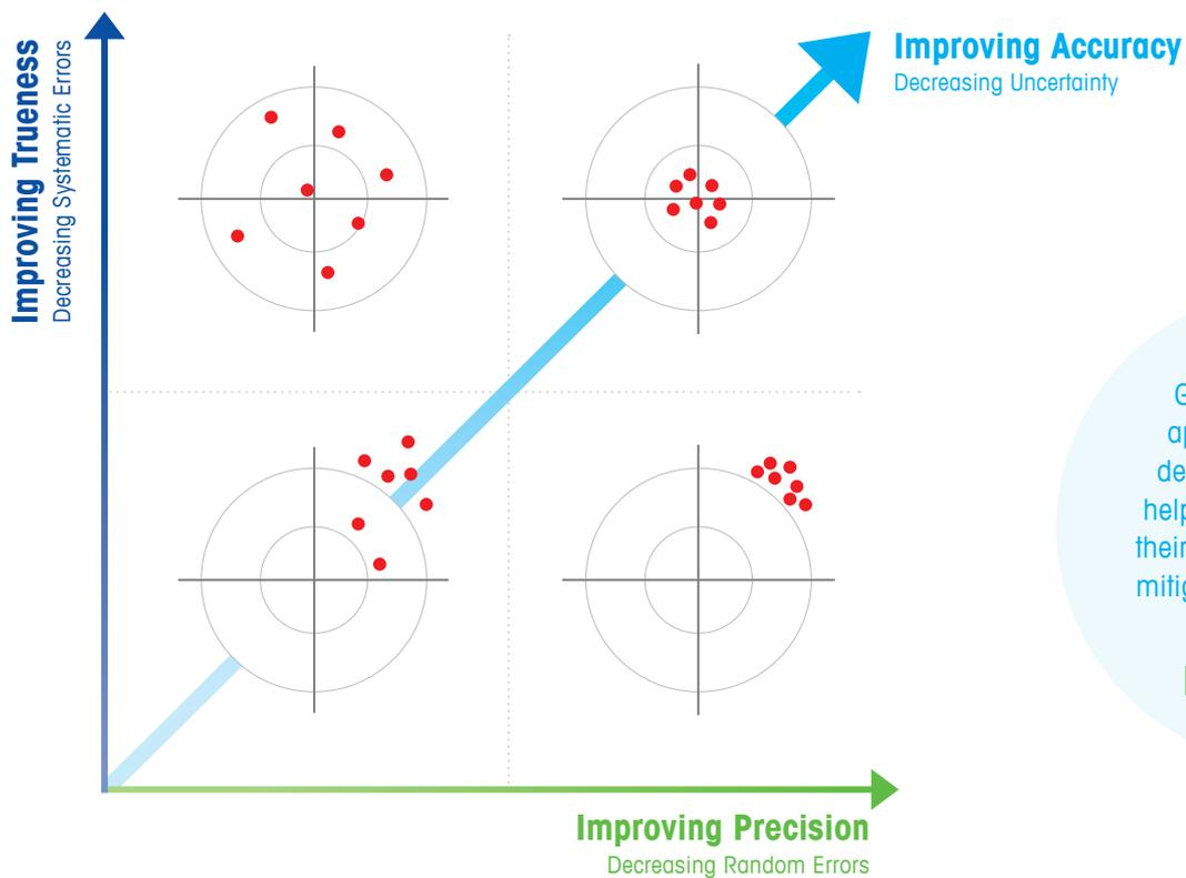
GPP is a systematic approach to pipetting developed by Rainin to help researchers improve their pipetting accuracy by mitigating both systematic and random error.
