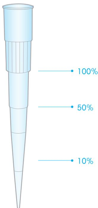
**Figure 12. Pipetting volume vs. range.** Rainin 200  $\mu\text{L}$  tip shown with 10%, 50% and 100% nominal volumes. Pipetting down to 10% can increase systematic error by as much as 2.5%.
