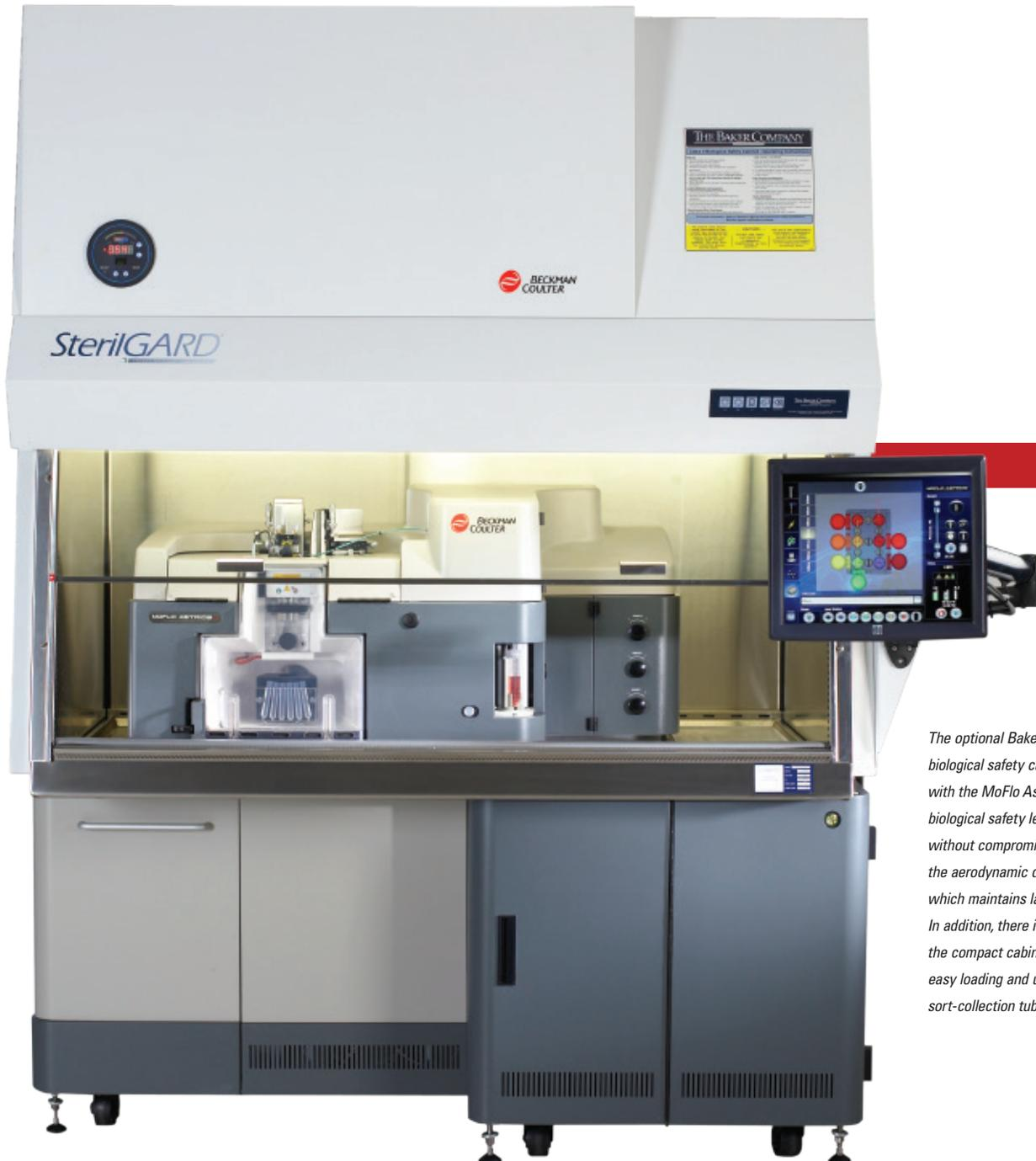
*The optional Baker Company SterilGARD biological safety cabinet can be fully integrated with the MoFlo AstriosEQ, to provide assured biological safety level BSL 2 containment without compromising workflow, thanks to the aerodynamic design of the AstriosEQ which maintains laminar flow in the cabinet. In addition, there is a convenient space within the compact cabinet for sample storage and easy loading and unloading of sample and sort-collection tubes, eliminating clutter.*
