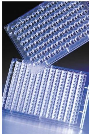
96 and 384 Well Protein Crystallization Microplates
