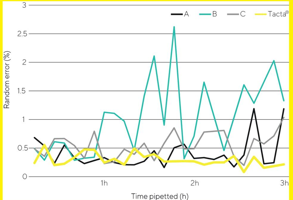
Precision of results tested over a three-hour period using four pipettes from various manufacturers. The test was performed by an independent laboratory in accordance with the ISO 8655 standard using 1000 µl pipettes with 1000 µl tips from the corresponding manufacturers.
