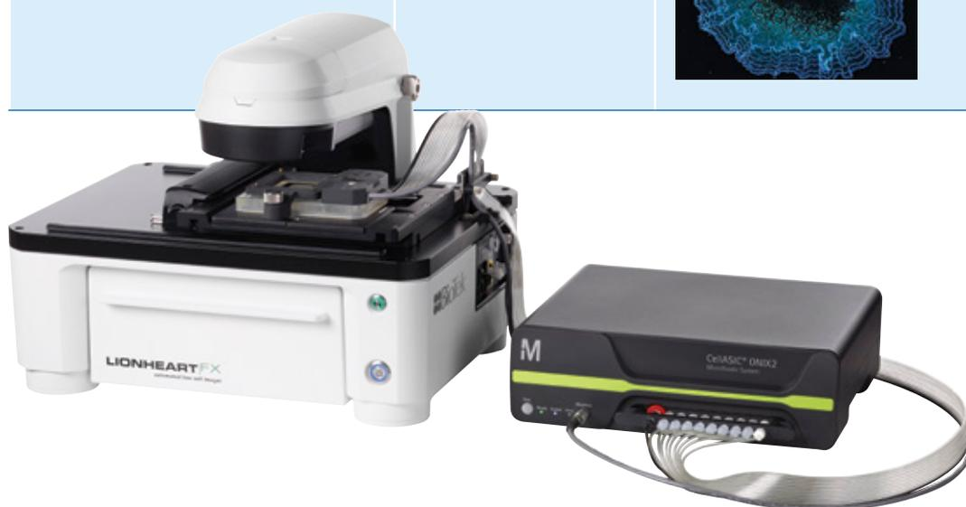
The CellIASIC® ONIX2 Microfluidic System works with your inverted microscope to enable long-term cell perfusion experiments and dynamic time-lapse analysis. (Shown with Lionheart™ FX automated Live Cell Imager from BioTek® Instruments)
