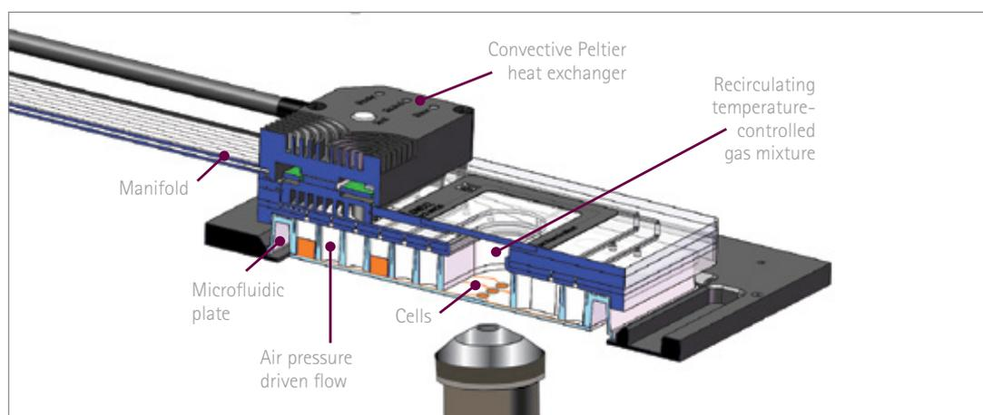
A low-profile manifold connects the control system with the microfluidic plates. Various manifold layouts are available to address different plate formats and application types.
