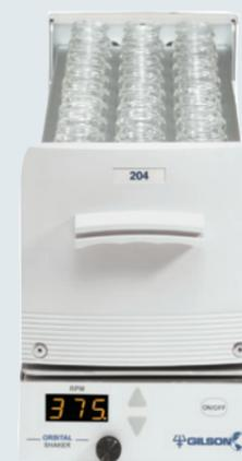
The Orbital Shaker is specifically designed for on-line or off-line liquid handling, vortexing, and mixing. It is a fully functional, stand-alone instrument. This compact shaker fits on one rack position of a GX-281 Liquid Handler bed. The shaker provides a range of customer-controlled shaking (20 to 720 rpm), allowing vortexing on various vessel sizes and sample volumes.
