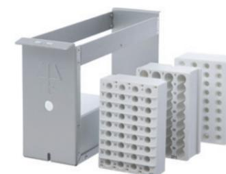
Gilson offers standard and custom SPE racks to meet the needs of any and all applications. A variety of vessels can be accommodated including tubes, vials, or microplates.
