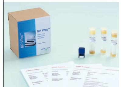
Our ready-to-use verification kit contains prefilled and sealed capillaries of three different certified reference substances, which are traceable to primary standards, for performance verification of your instrument.
