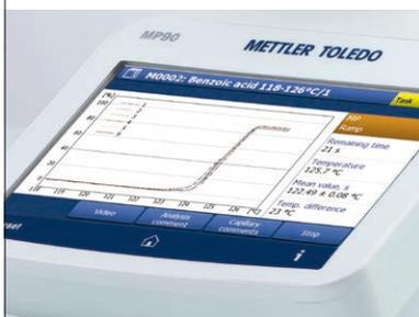
Automatic detection of transmitted light combined with video observation ensures that the melting, slip melting, boiling, and cloud point measurements are reliable. Statistical evaluation with standard deviation and mean value allow you to have full confidence in your data.
