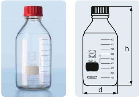
DURAN® original GL 45 Laboratory Bottles are available complete with high temperature screw caps and pouring rings. The PBT cap and ETFE pouring rings offer greater thermal and chemical resistance than the equivalent polypropylene components.
