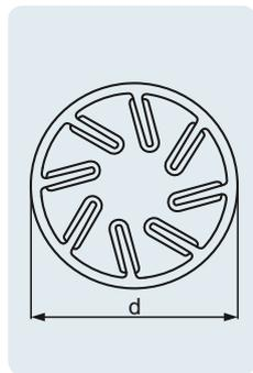
The holder helps stabilise bottles during activities such as liquid dispensing or pipetting. The flexible ribs accommodate both round and square bottles with diameters or base widths of between 75mm and 120mm. The solid silicone construction makes the holder autoclavable, durable, and chemically resistant.
