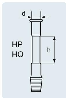
Ground and polished bearing surface, with standard ground cone.
