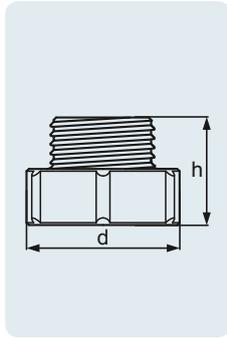
The re-usable adaptor (GL 45 external / GL 56 internal) allows the use of the DURAN® TILT bottle with 45 mm filtration units for the filter sterilisation of cell culture media. Manufactured from inert PTFE; can be autoclaved and depyrogenised at 300 °C.
