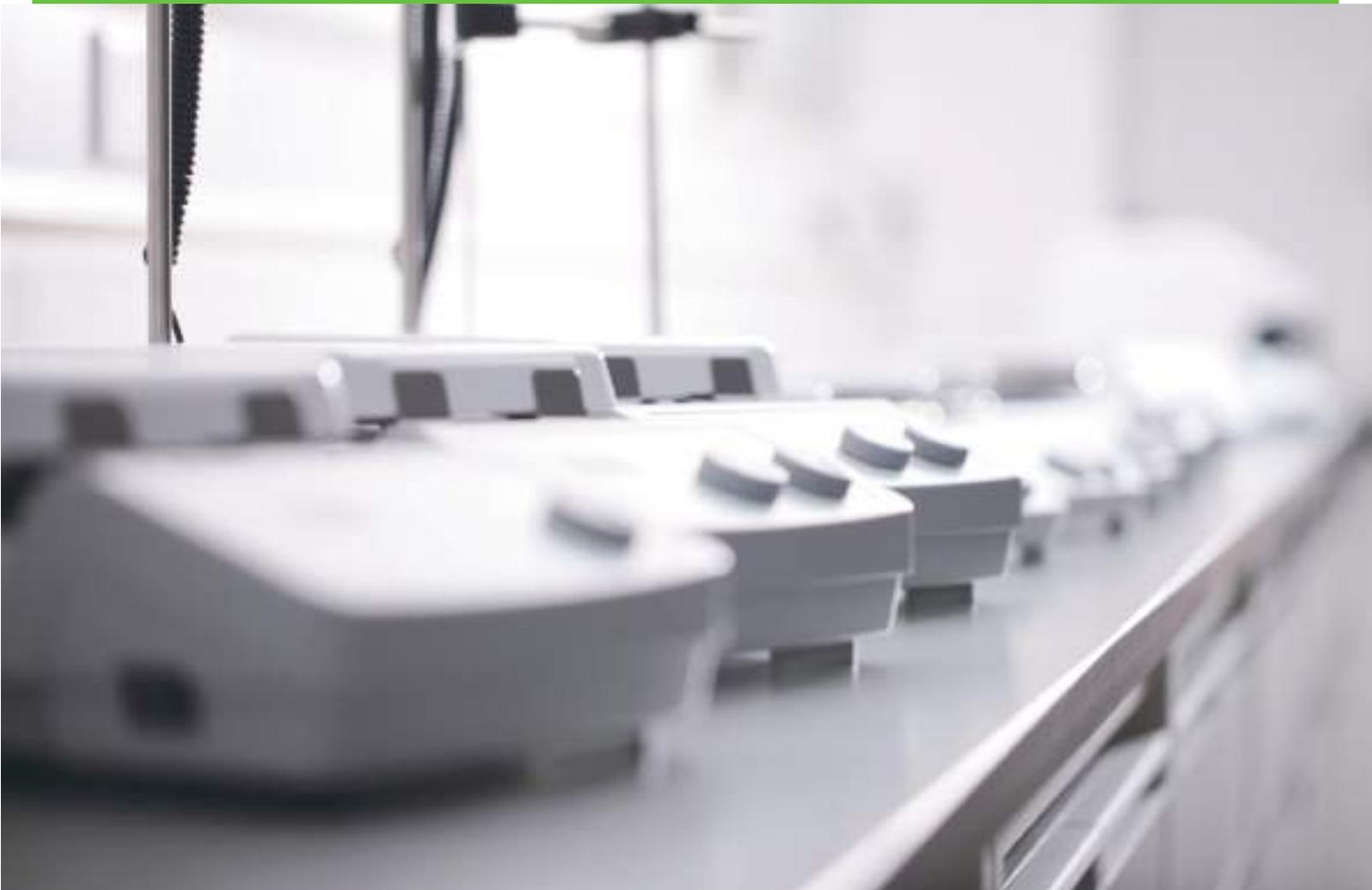
Magnetic hotplate stirrers are used for low viscosity liquids or solid mixing, widely used in chemical synthesis, physical and chemical analysis, bio-pharmaceuticals etc. DLAB provides different series, heating range covers from 120°C-550°C:
