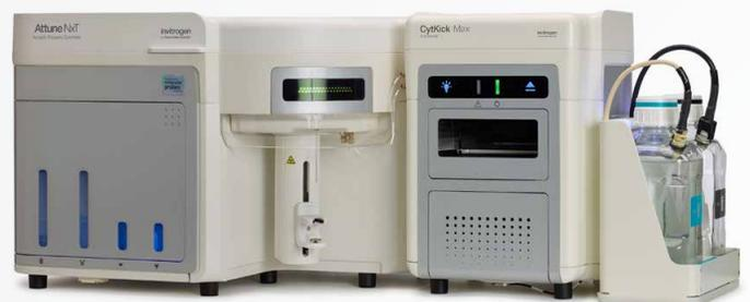
Figure 11. Umbilical cords connect the Attune NxT Flow Cytometer and the Attune NxT External Fluid Supply.
