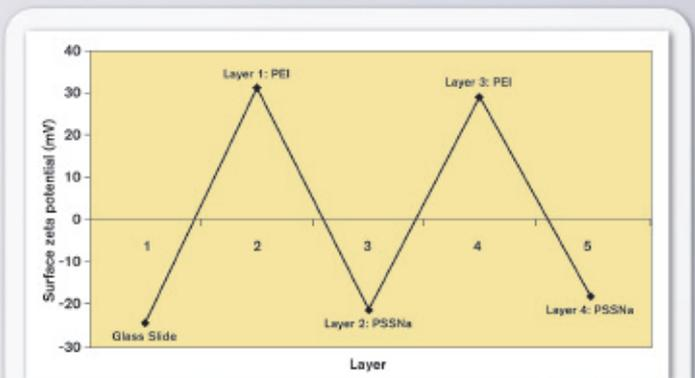
Zeta potential of glass slide coated with PEI and PSSNa polyelectrolytes layer by layer (LBL) alternatively.
