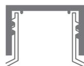
**Phenolic-style caps** are designed (when loosened) for use in open systems requiring gas exchange. With the caps slightly loosened, gas is exchanged between the environments inside and outside of the flask.
