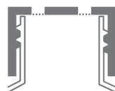
**Vent caps** contain a 0.2 µm pore, hydrophobic membrane sealed to the cap, isolating the container it is placed on from the environment while providing consistent gas exchange. These caps are highly recommended for use in all CO<sub>2</sub> incubators, especially for long-term use. The vent cap was a Corning innovation that first appeared in 1988.
