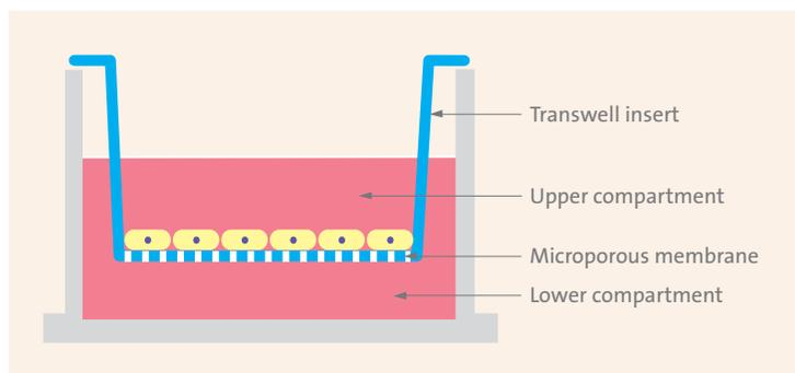
The unique, self-centered hanging design of Transwell inserts prevents medium wicking between the insert and outer well. The design also permits access to the lower compartment through windows in the insert wall, as well as undamaged co-culturing of cells in the lower compartment.
