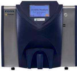
Use a simple, yet accurate solution for moisture tests. UGMA compliant impedance measurement at 149 MHz gives a representative moisture analysis of the whole kernel. A result for test weight is delivered simultaneously. Test hot or frozen grain within a wide temperature range from -20 to +45°C. It is fully-connected via the FossManager™ networking software that supports grain networks around the world.
