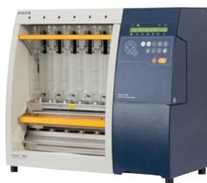
This is a fully automatic system that uses internally preheated reagents added to a closed system to minimise contact with hot reagents. It determines fibre content according to Weende, van Soest and other recognised methods. Single or sequential extractions including boiling, rinsing and filtration are performed under reproducible and controlled conditions.
