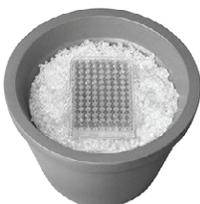
Plate directly on crushed ice, the plate does not reach 4°C in any of the wells and well-to-well temperature is uneven.
