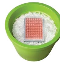
Plate placed on Corning CoolSink module and then placed on ice shows more uniform well-to-well temperature and all wells at or below 4°C. (Blue center plate wells are slightly warmer due to curvature of the underside of the plate).
