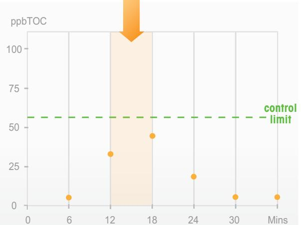
**At-line Batch Analyzer** - Batch measurement, 6+ minutes
