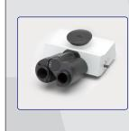
Super wide field of view (FN 26.5) trinocular tube with fixed 24° inclination and interpupillary distance adjustment. Light partitioning selector (Binocular/ Camera: 0/100, 100/0, 20/80).
