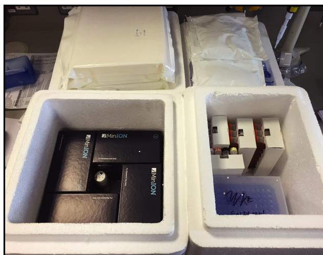
20 samples. MinION sequencing requires a mix of chilled and frozen reagents. Recommended shipping conditions are specified. The picture underneath depicts MinION flowcells ready for shipping with insulating material (left) and frozen reagents (right).
